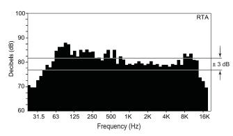
Figure 1: On-axis frequency response.
