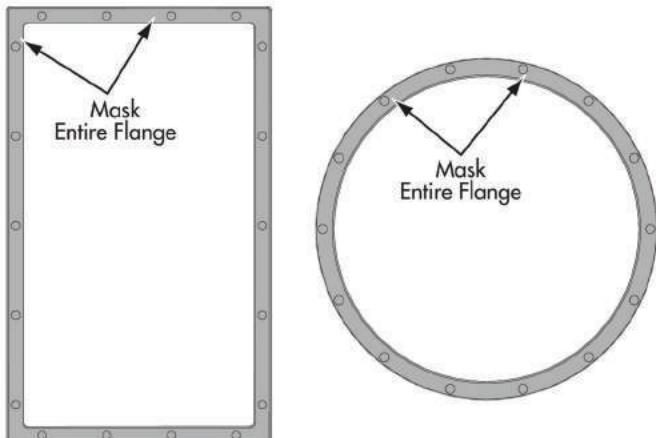
FIGURE 1: MASK THE FLANGES OF INSTALLED VP SPEAKERS BEFORE PAINTING THE WALL OR CEILING
