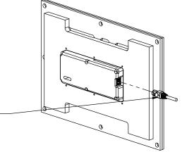
If required, it is possible to unscrew 6 screws, remove the back wall and connect POE cable after the wall mount was installed.
