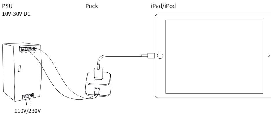
The cable between the DC power supply and the Puck must have a cable section of at least 0.8mm<sup>2</sup> and maximum 1.5mm<sup>2</sup>. The applicable maximum cable lengths are specified below:
